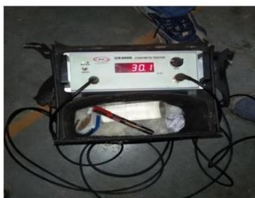
Fig 19: Test of bacterial concrete samples using Ultrasonic Pulse Velocity Machine.
