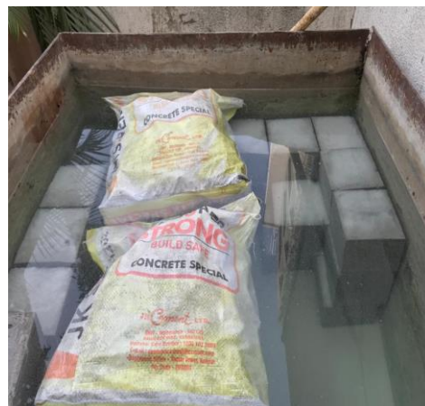
Fig 7: Curing of cubes
