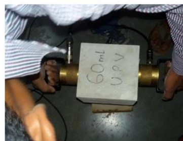
Fig 19: Test of bacterial concrete samples using Ultrasonic Pulse Velocity Machine.
