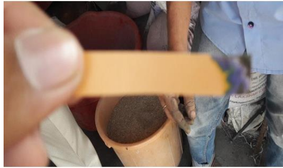
Fig 11: Litmus paper indicating the pH value of Concrete
