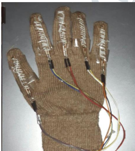
Fig. 3. Flex sensor Implemented on fingers.
