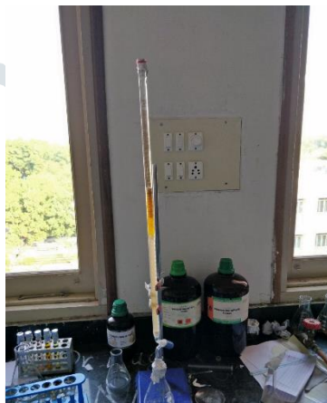
Fig.1: Column chromatography of Chalcone derivatives
