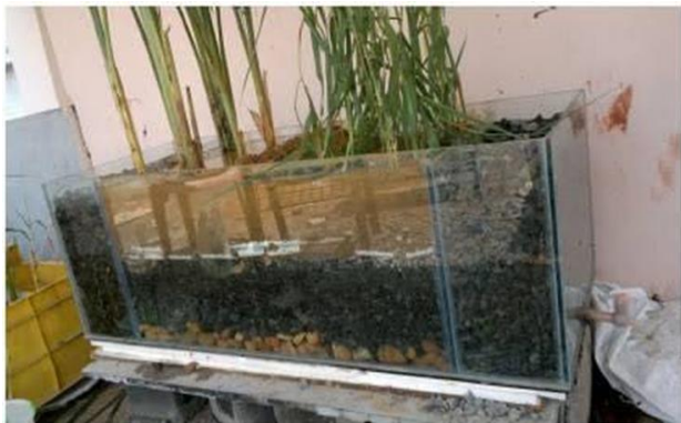
Fig 4.3 Design of horizontal flow constructed wetlands
