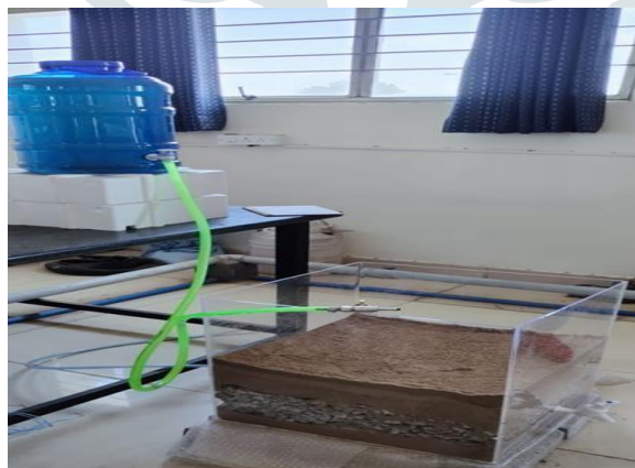
Fig 4.2 Design of vertical flow constructed wetlands
