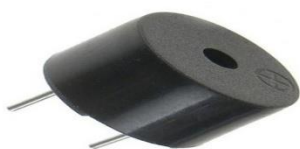
Figure 9: Buzzer used with Raspberry Pi
