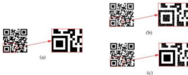
Fig.1 Comparison of standard QR Code(a), with (b)proposed private QR code for private message sharing and (c)proposed code for authentication
