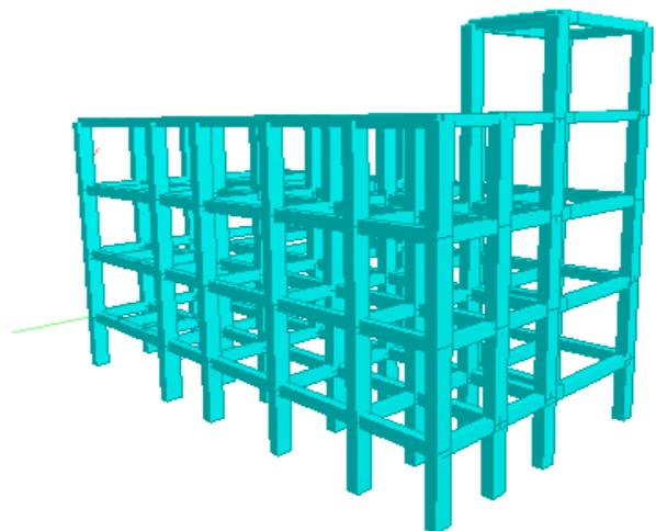
**Fig. 2: 3-D view in STAAD.Pro without floating column**
