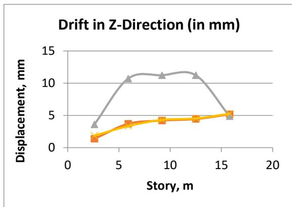
**Fig. 8: Maximum Story drift of the floating column at Z-Direction**
