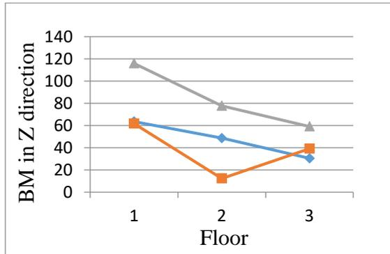
**Fig. 11: comparison graph of Bending moment for all models**
