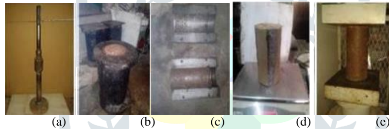
Fig. 1. Sequences involved in preparation and testing of cylinder specimens (a) Tamper used for compaction of cylindrical specimens, (b) Cylindrical mould of 102 mm diameter and 203 mm height used for compaction, (c) Removal of specimen from the mould after 24 hours, (d) Weighing of specimen after proper sealing, (e) Curing of specimens in the BOD incubator at a constant temperature 23.7°C
