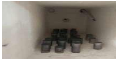
Figure 9 Pellets in Muffle Furnace
