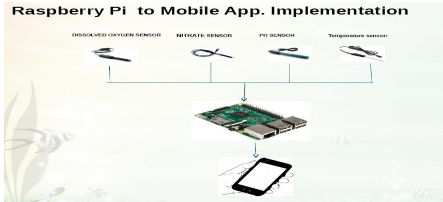
FIG 3.CONNECTION BETWEEN SENSORS TO PI TO MOBILE
