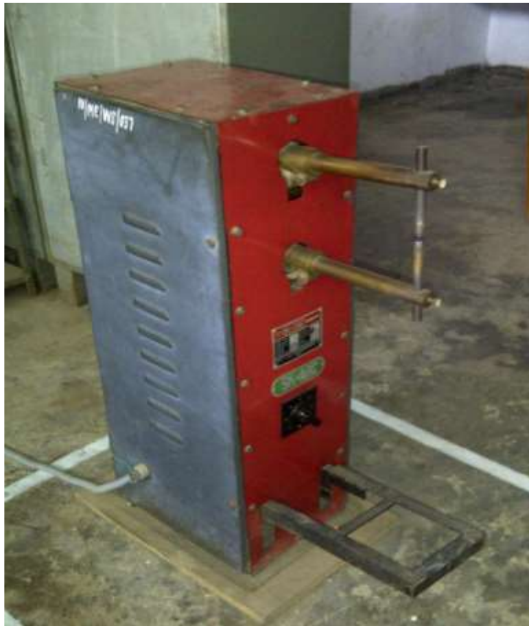
Figure 4.2 Picture of spot welding machine used for experiment
