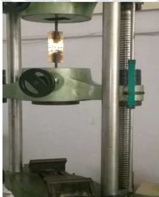
Figure 4.3 Picture of tensile strength evaluation by UMT machine
