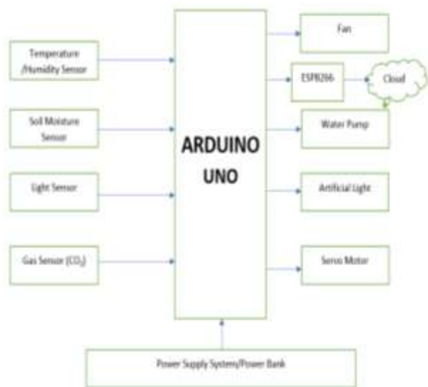
Fig. 2. Architecture of the proposed system
