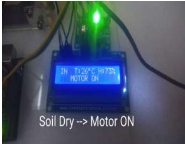
Fig.18: shows motor ON condition when soil dry
