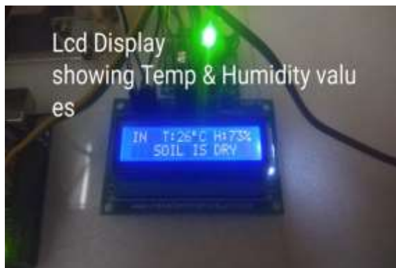
Fig.16: Temperature and humidity values displayed on LCD when setup working condition
