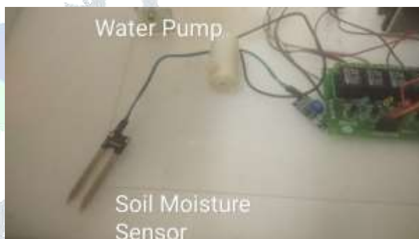
Fig.15: Water pumps and soil moisture sensor in setup
