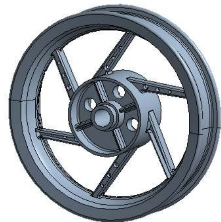
Fig. 10. Optimized design of wheel
