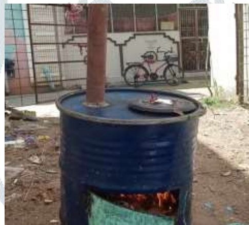
Figure 4: Burning of waste in the incinerator
