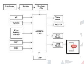
Fig: BLOCK DIAGRAM OF PROPOSED SYSTEM
