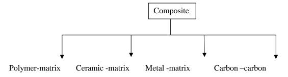
Fig.1.8: Classification of composites on the basis of matrix [1, 5]
