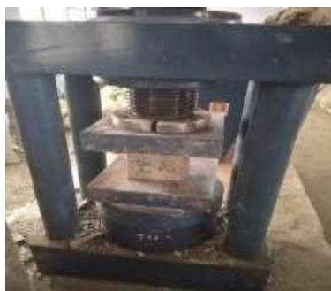
Fig.3: Compressive Strength test.
