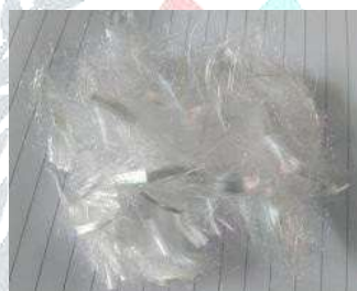
Fig.1 (b): Polypropylene fibre
