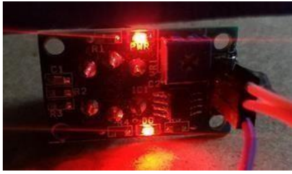
Fig.10 MQ2 sensor indicating detection of gas
