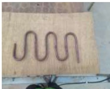
Fig.3. U shaped copper coil
