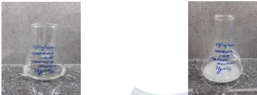
Figure 1: color change indicates the formation of nanoparticles
