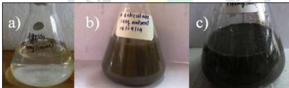
Fig. 1. Color change during the phyto-reduction Ag + to Ag NPs, white to brown after 24 h. incubation. a) AgNO 3 b) A. reticulata leaf extract c) AgNO 3 with leaf extract.
