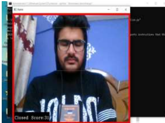
Fig3: Red box as eyes detected closed
