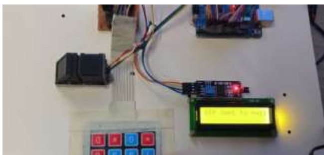
Fig.10: LCD showing that the OTP sent to mail after entering the password
