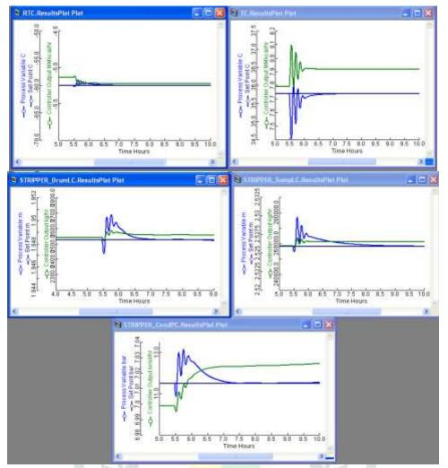
From the above response it is observed that in recycle temperature controller, temperature of the recycle stream varies suddenly and then reaches steady state. It increases gradually and slowly reaches steady state because of sudden increase in feed flow. Because of increase in feed flow, column reboiler duty increases along with drum and sump levels as the pressure also increases. But all other controllers fisrt decreases with step uop change and increases slowly and reaches steady state.
