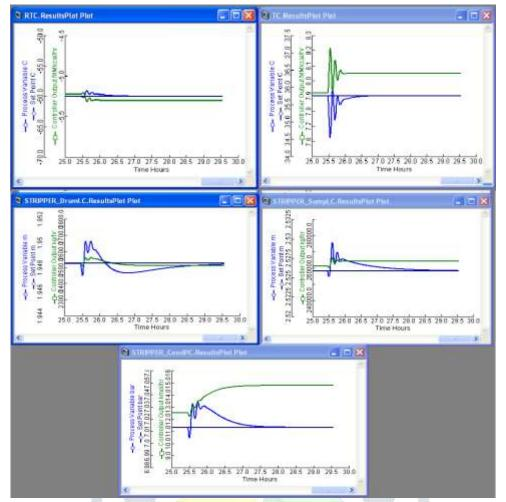
From the above plot, its clear that after reaching the steady state with a disturbance initially, controllers responds fast and takes less time to reach steady state in order to compensate the disturbance. The responses are similar to the previous steu change but with quicker action to reach steady state.
