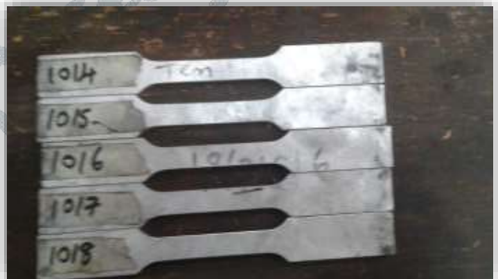
Figure.8: Tensile test specimen prepared as per ASTM (E8) Standard
