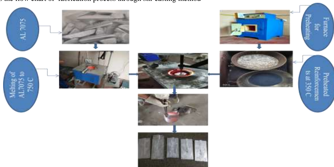
Figure 2: Flow chart showing Stir casting procedure involved preparation of MMCs
