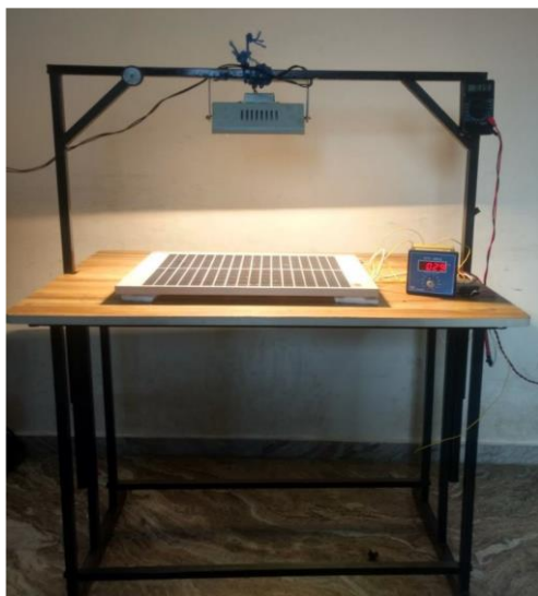
Figure 2 actual photograph of experimental set-up shows an experimental setup without cooling.
