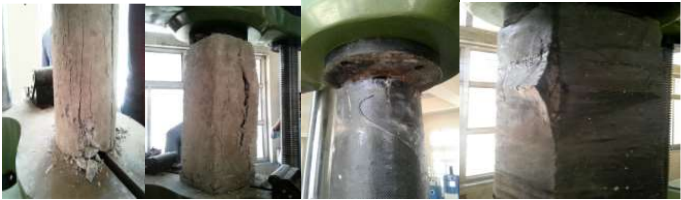
Figure 6.1.4.2: Mode of Failure of CFRP Wrapped Columns
