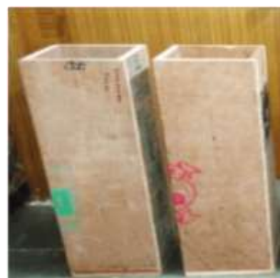
Figure 6.1.1: Rectangular Mould Having 200 X 230X700 mm ,Square-200X200mm
