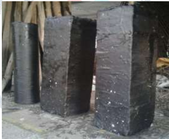
Figure 6.1.3: Applying Epoxy Resin and Wrapping CFRP on Specimens
