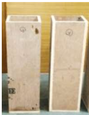
Figure 6.1.1: Rectangular Mould Having 200 X 230X700 mm ,Square-200X200mm
