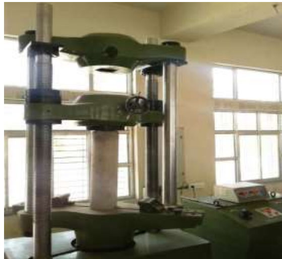
Figure 6.1.4: Universal Testing Machine Having 100 Ton Capacity
