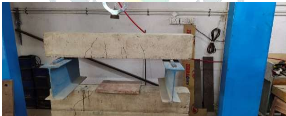
Fig-1: Crack pattern observed form normal beam
