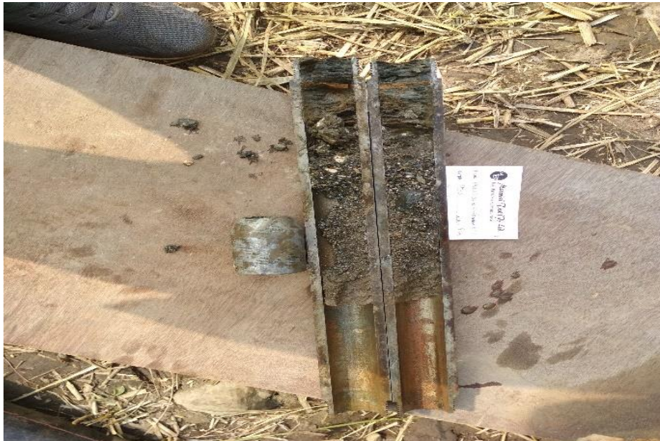
Figure 2: Split Spoon Sampler (SPT sample)
