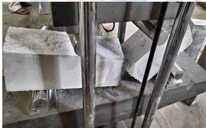
Fig 12. Testing of prism specimen in the laboratory under two-point loading
