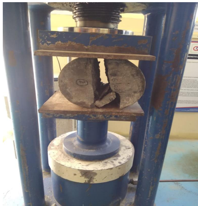
Fig 8. Testing of cylindrical specimen in the laboratory under compression testing machine
