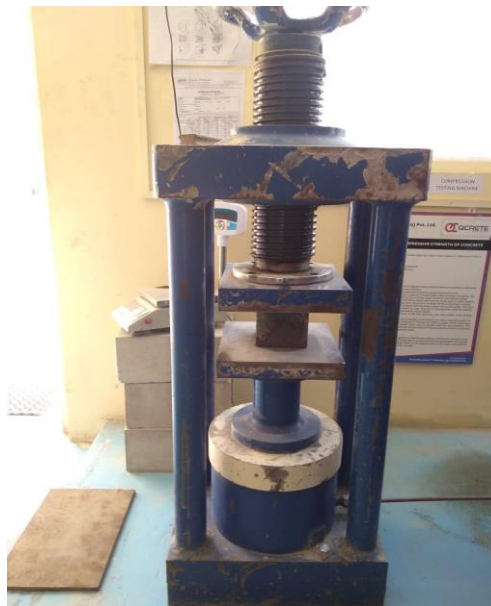
Fig 4. Testing of cubical specimen in the laboratory under the compression machine
