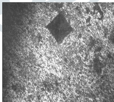
Fig. Impression made by indenter on surface of insert
