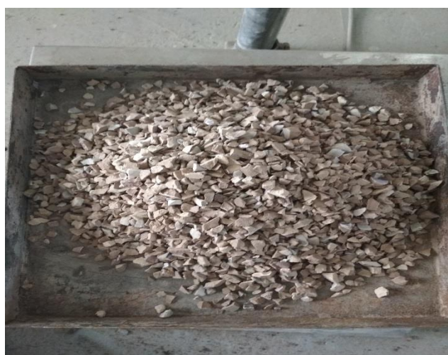
Fig.2. Ceramic Waste tile aggregate
