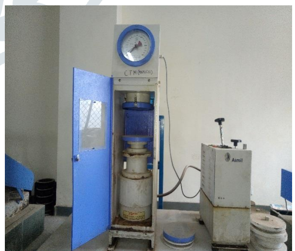
Fig.5. Compressive strength testing machine
