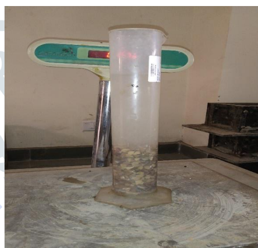
Fig.3. Water Absorption of waste tile aggregate
