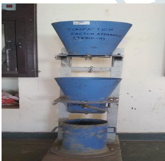
Fig.4. Compaction factor test apparatus
