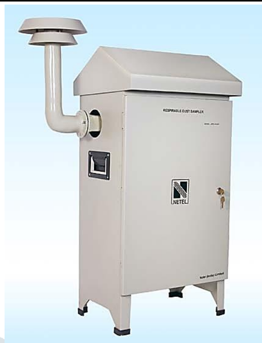
Fig. 3: Equipment used in analysis PEM-HVF-1/110 & NPM-HVS
