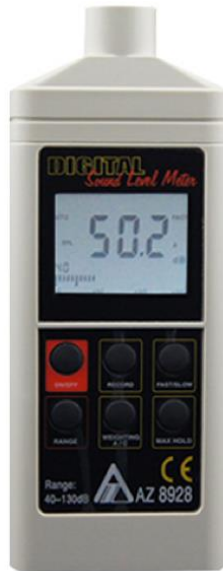
Fig. 8: Equipment used in the analysis CE 8928 digital sound meter
