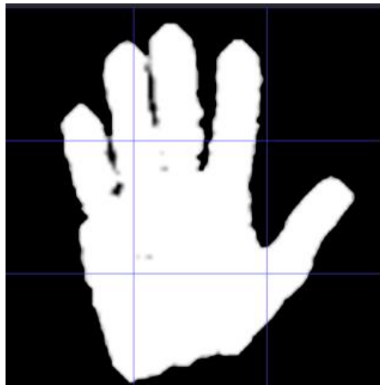
Fig (4): the ISL hand pose fragmented by a 3x3 grid.
