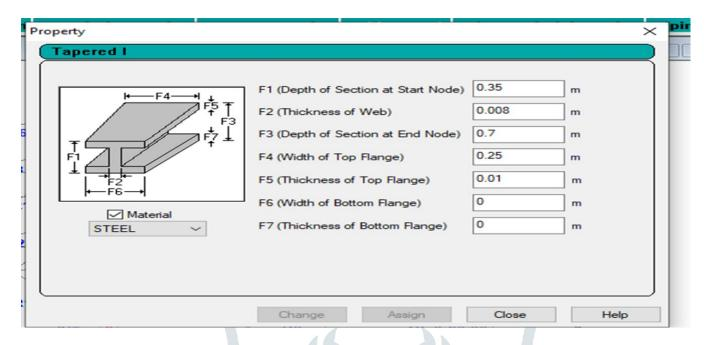
It is observed that the weight of the tapered section is around 30% less than that of the conventional steel structure.
