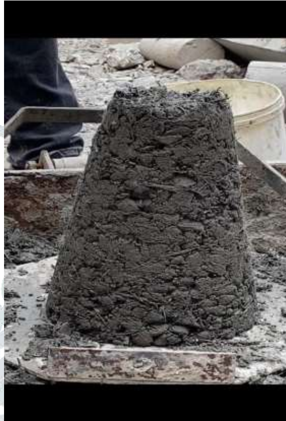
(True slump formed in one of the mixes)
