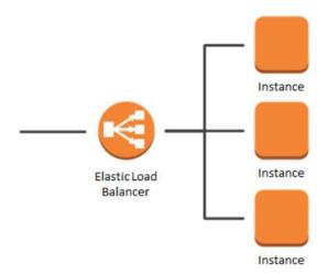
A load balancer distributes the incoming application or network traffic across multiple targets, such as Amazon EC2 instances, containers, and IP addresses, in multiple Availability Zones. It uses health checks to detect which instances are healthy and directs traffic only across those instances.
