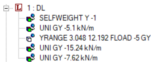
Figure 3.2.1.2: Dead Load Intensity Applied on the Building
