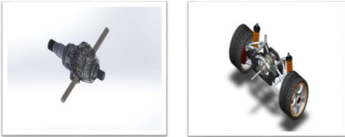
Figure 2 – (A) Orthogonal view of Differential (B) Orthogonal view of Rear axle
