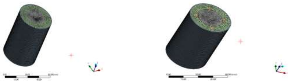
fig 9:Meshing for BTMS with non-accessible fin structure fig 10:Meshing for BTMS with accessible fin structure
