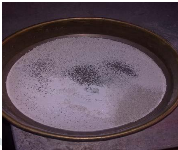
Figure 8 – Soil sieve apparatus.
