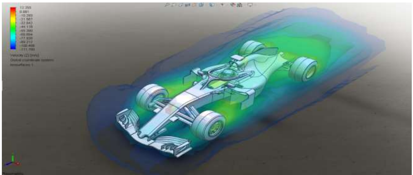
Fig.22 Velocity isosurface of model in isometric view
