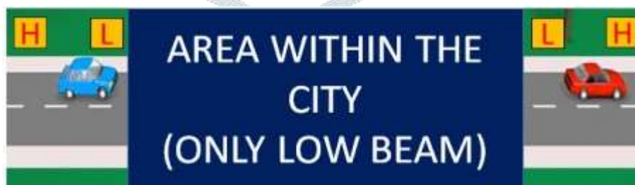
Fig. 4. – Automatic high to low beam switching and vice versa when crossing city limits [14].
