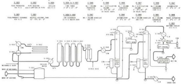
Conventionally, the aldol condensation of acetone is conducted using a homogeneous base catalyst such as methanolic NaOH or KOH giving acetone conversion of around 12%. In the conventional process, citric acid is added to neutralize the catalyst and stabilize DAA, after which DAA is recovered by evaporation, and by stripping off the acetone, it is then recycled.
