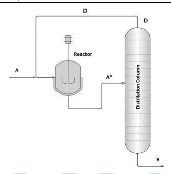
RDR process consists of two main units namely Reactor and a distillation column. Barium Hydroxide Ba (OH)2 is used as the catalyst. The diacetone alcohol is accumulated in the distillation still until the required concentration is reached.
