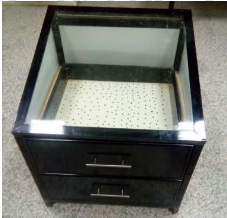
Fig. 1 Photograph of solar dryer made by students
