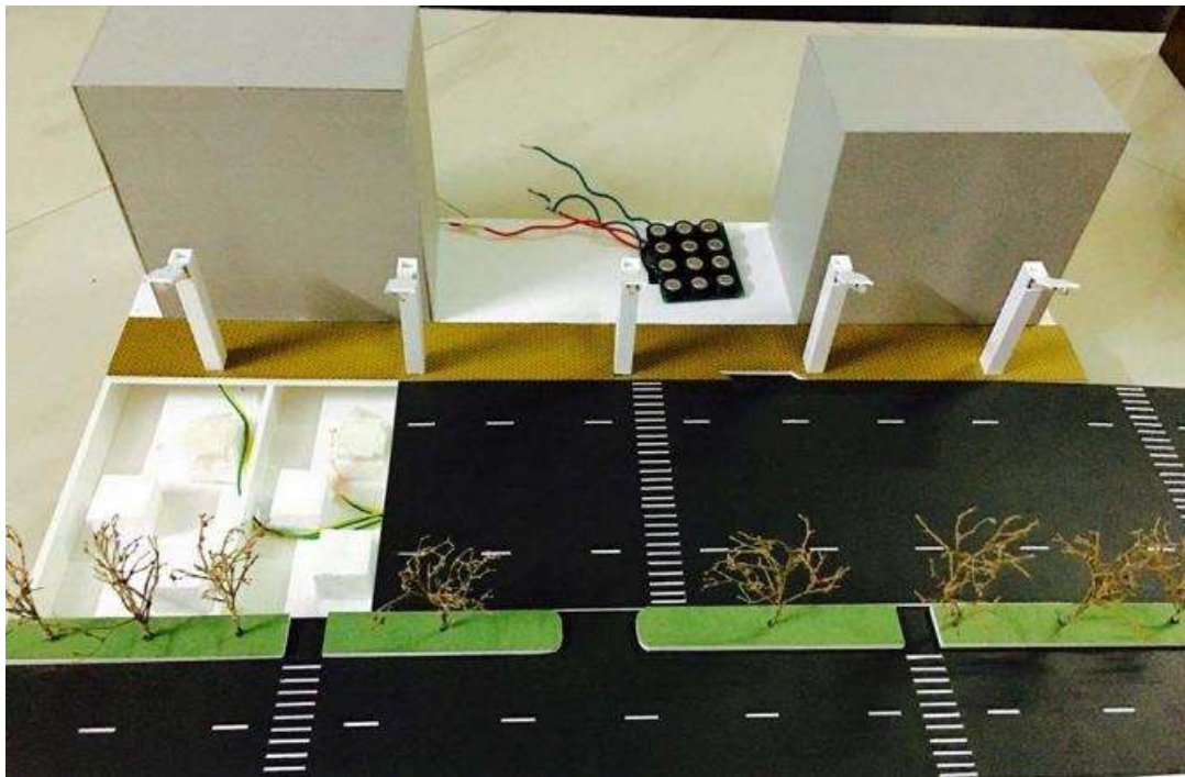
Fig (5) The prototype smart street lighting system where the piezo materials are placed under the slabs of the road.
