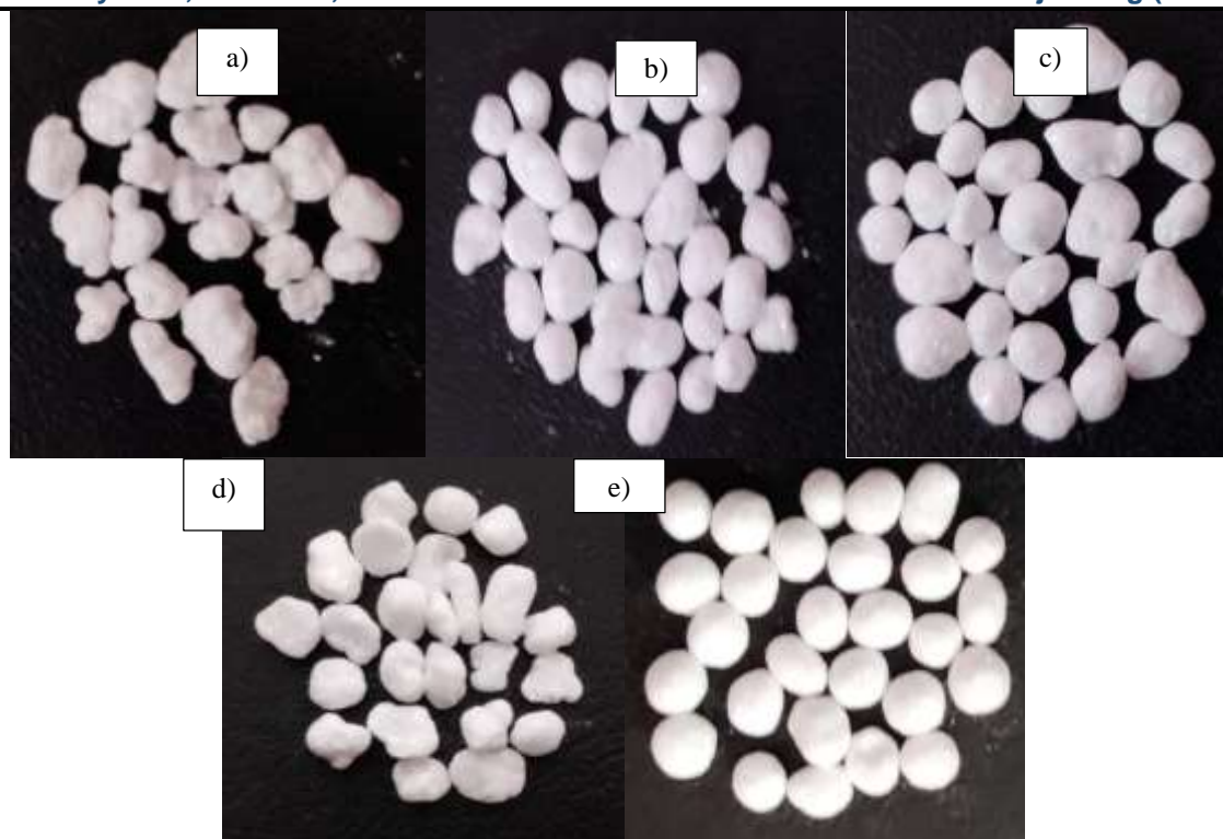
Figure 8: Particle morphology at different times (a) 5min (b)10 min (c) 20 min(d) 45 min (e) 60 min Benzoic acid conc. = 0.375 g/ml, N=600rpm, BSR=1, size= 1 mm
