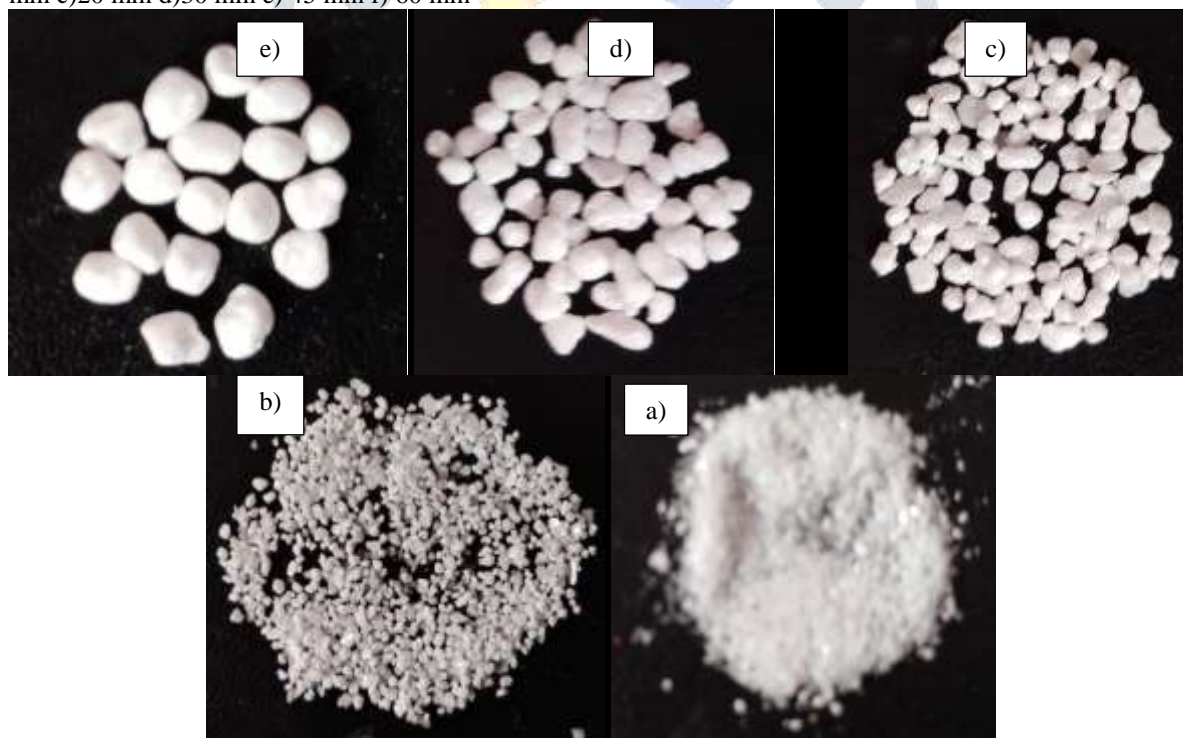
Fig.7. Particle morphology of different sieve fractions (a) 0-355 \mu\text{m} (b) 355-600 \mu\text{m} (c) 600-1000 \mu\text{m} (d) 1000-1400 \mu\text{m} and (e) 1400-2000 \mu\text{m} . Benzoic acid conc. = 0.375 g/ml, N=600rpm, BSR=1, Time at 45 min
