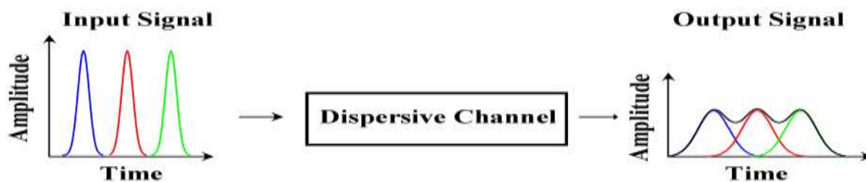
Fig 3: Pulse broadening caused by dispersion
