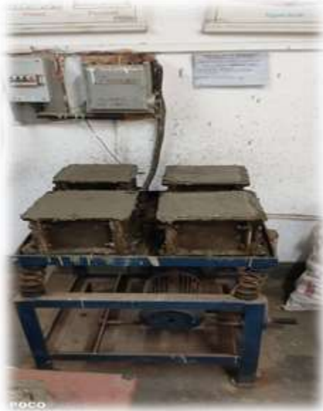
Compaction By Vibration
