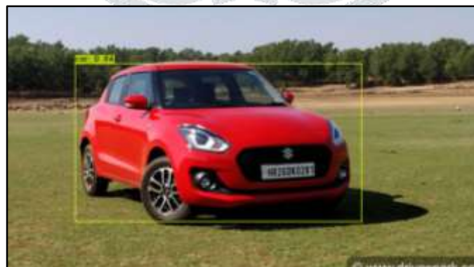
Figure 3.2: Bounding Box drawn using the co-ordinates given by YOLO detection
